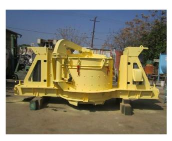
Cemco Turbo Vertical Shaft Impact Crusher KDEV80
