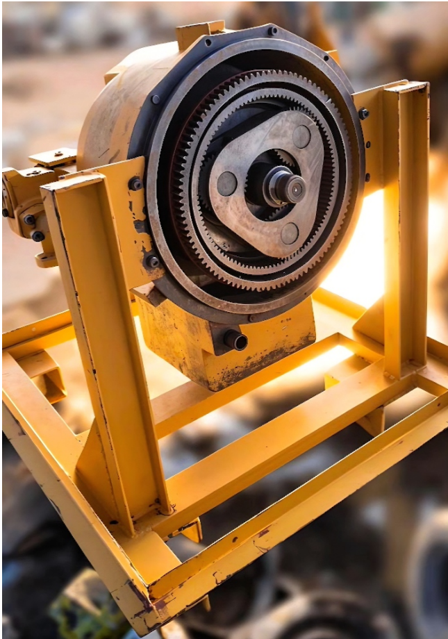
CAT D9R Torque Converter
