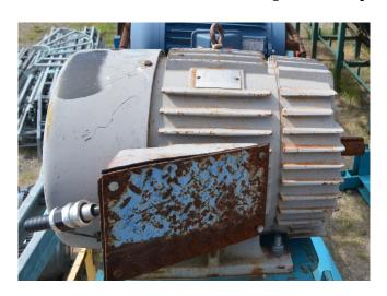
Horsepower: 40Voltage: 575RPM: 3555Frame: 324TS
