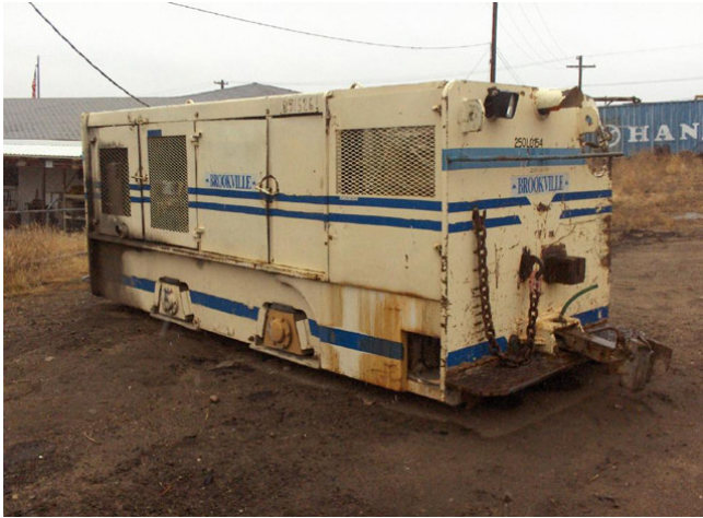
Brookville 15 Ton Locomotive. 36 in. Gauge. Diesel Driven.
