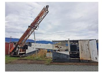
Savona Equipment ltd. is offering a Boart Longyear diamond core drill package that includes 1 x Boart Longyear 50 and 1 x Boart Longyear 38 that are both skid mounted. Each drill comes with a half shack on skid with mud tanks and mixers.
