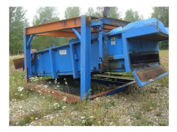
BM&M 2-Deck Inclined Shaker Screen
