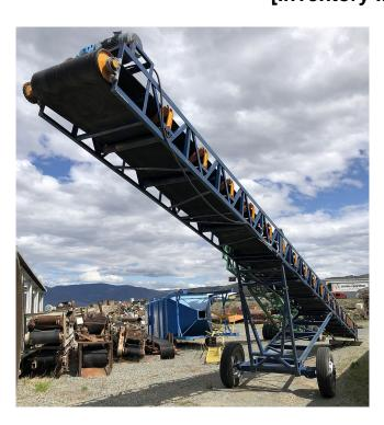
Better 36in x 60ft Chassis Mounted Radial Stacking Conveyor
