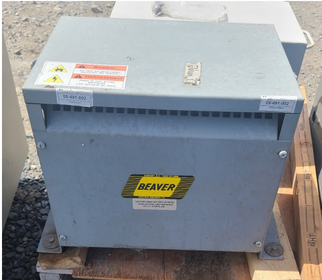
Beaver 15kVA Transformer
