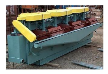
Bank of 6 Denver # 15 Flotation cells. Unit was supplied refurbised and ready to install.
