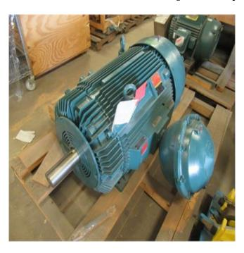
Voltage: 600 VoltExplosion ProofRPM: 1188
