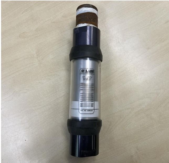
AW-Lake G5A4AM99 Pneumatic Flow Meter
