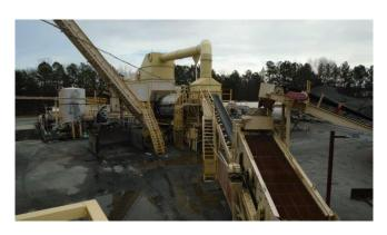
Astec Semi-Portable Counterflow Asphalt Plant
