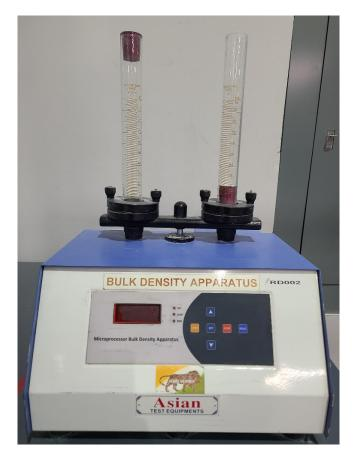
Asian Test Equipment Bulk Density Apparauts
