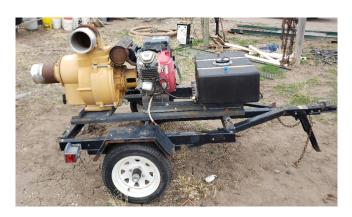
• Maximum Solids Handling Capacity: 3 in. Dia.
