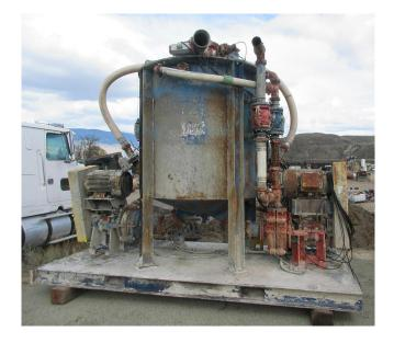
Amix 4000 Liter Colloidal Mixer Grout Plant
