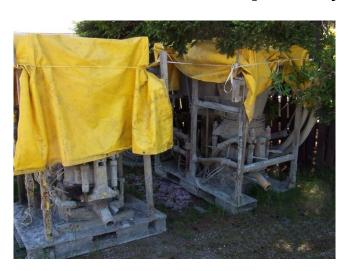
The Aliva 252 is a sturdily constructed skid mounted concrete spraying machine for the processing of dry mix.
