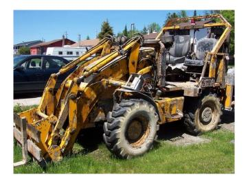
Complete Shotcrete package of Miller JCB Triple 4CE Carrier with Hiab Boom, En-Creter attachment, and 2 - Aliva 252 Shotcrete Machines.
