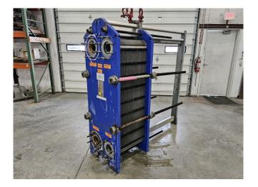
Alfa Laval Gasketed Plate-and-Frame Heat Exchangers
