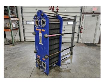
Alfa Laval Gasketed Plate-and-Frame Heat Exchangers
