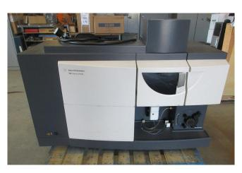
Agilent 700 Series ICP Optical Emission Spectrometer
