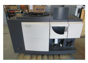
Agilent 700 Series ICP Optical Emission Spectrometer
