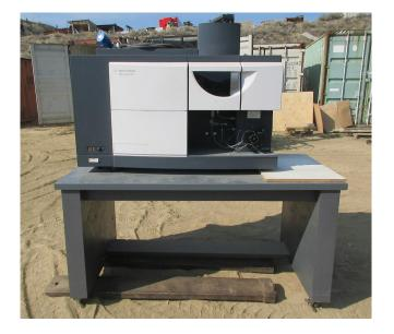
Agilent 700 Series ICP Optical Emission Spectrometer
