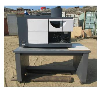
Agilent 700 Series ICP Optical Emission Spectrometer
