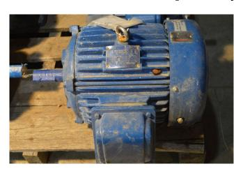
HP: 7.5Volts: 575RPM: 1755Frame: 213T
