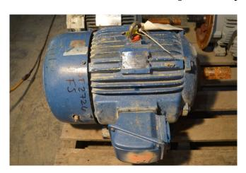
HP: 25Volts: 575RPM: 1765Frame: 284T
