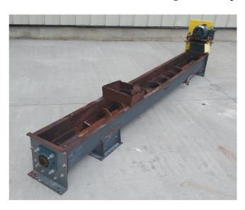
9in Dia. x 10ft Long Center-Feed Auger
