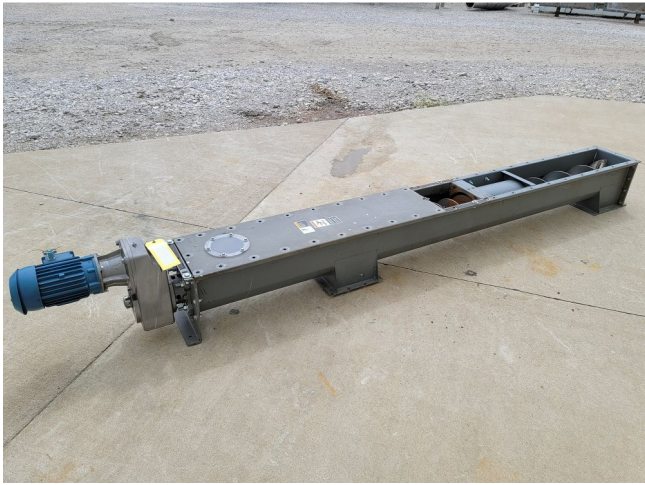
9in Dia. x 10ft Long Auger
