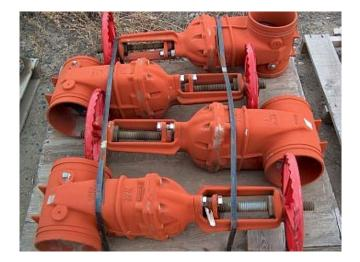
8 inch gate valves. Victaulic groove ends with rubber coated gate and poly coated housing
