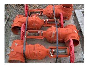
8 inch gate valves. Victaulic groove ends with rubber coated gate and poly coated housing
