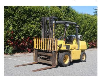
Max. Lift Capacity: 8,000 lbs.Max. Lift Height: 194 in.
