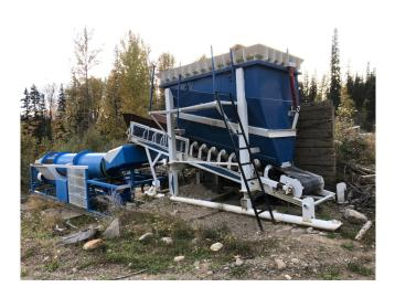
This Scrubber Trommel Wash Plant has a max capacity of approx.. 75 YPH. It comes complete with a Grizzly Hopper Feeder, Feed Box, Scrubber Wash Drum with Trommel Screen, Sluice Box, and Discharge Belt.
