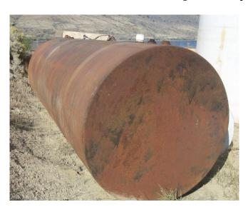
7 ft Dia. x 21 ft 5,000 Gallon Steel Tank. Very Good Condition.
