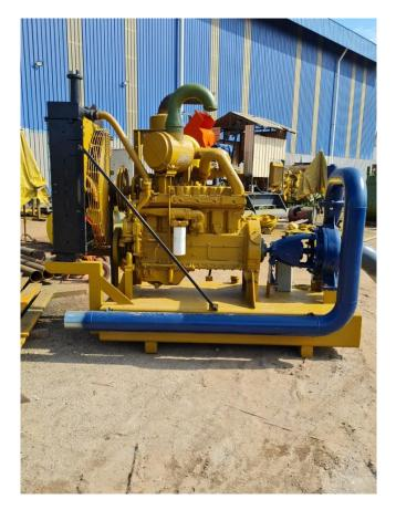
6x8 Centrifugal Pump with CAT Engine
