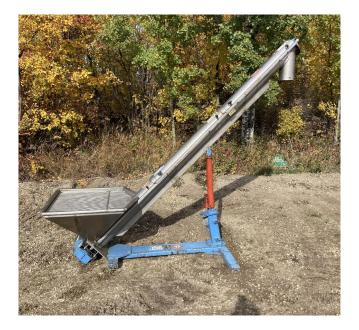
6in Dia. x 10ft Stainless Steel Auger
