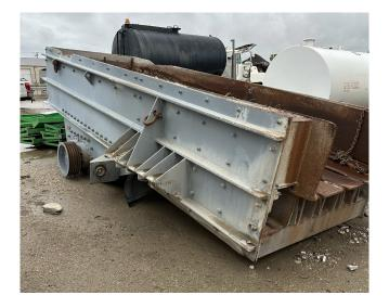
6ft x 12ft Vibrating Pan Feeder
