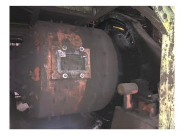
6ft Dia. x 4ft Hardinge Conical Ball Mill
