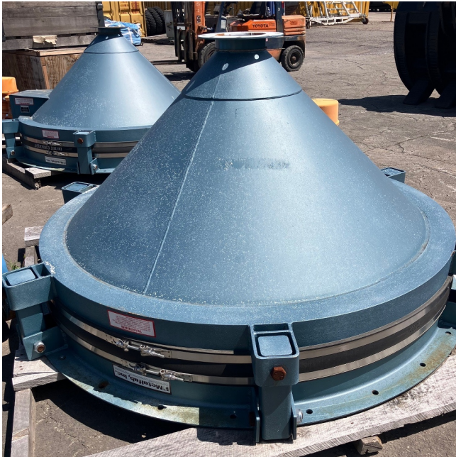
6ft Dia. Metalfab Bin Activator
