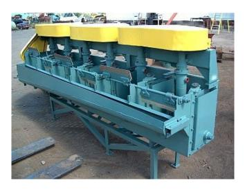
6 Used Denver Flotation Cells. Bank of #8 Sub As. Units supplied refurbished.
