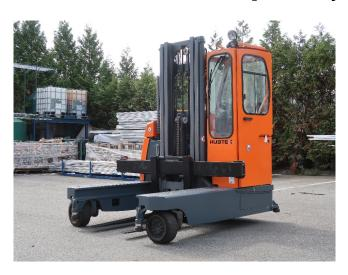
Max. Lift Capacity: 6,600 lbs.Max. Lift Height: 216 in.
