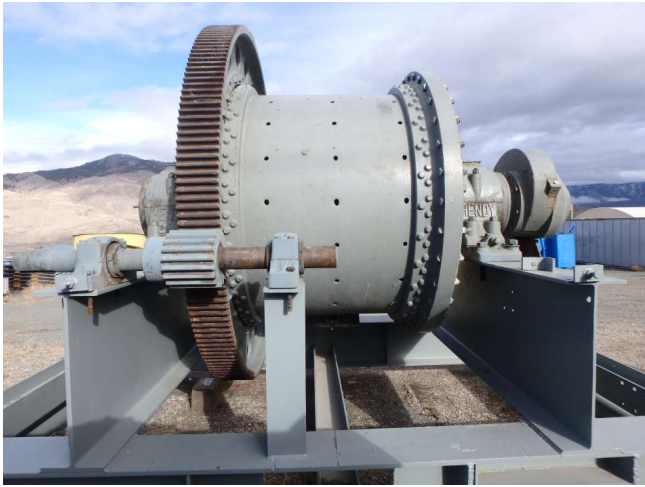
5ft Dia. x 4ft Long Ball Mill
