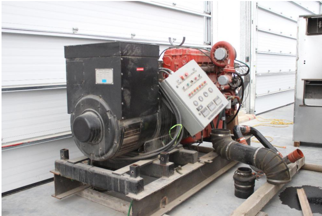
500kW Cummins QSX15 Diesel Generator
