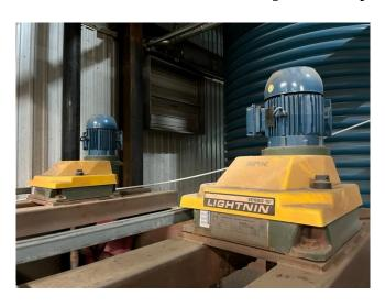
5,264L Stainless Steel Tank with Lightnin Agitators
