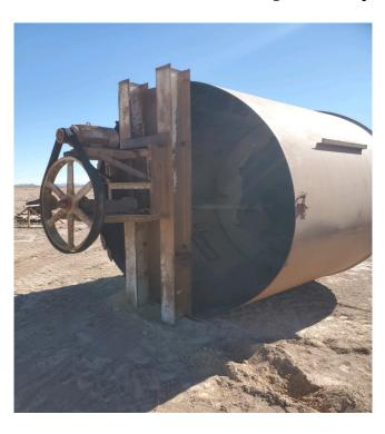
4500 Gallon Mixing Tank with 10HP Agitator
