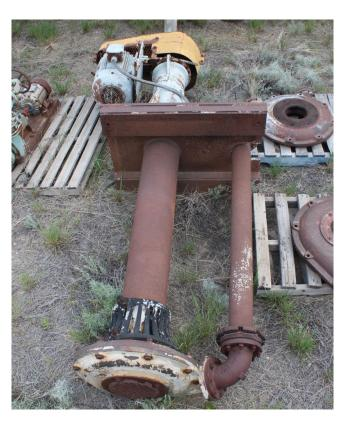
4 in. Galligher sump pumps x 72 in. depth(Can be converted to a 6 in.)
