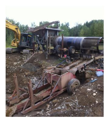
4 ft. x 16 ft. Trommel Complete with Sluice and Hopper. Driven by 11 HP Honda Gas Motor.
