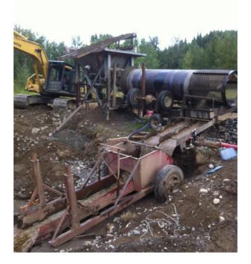
4 ft. x 16 ft. Trommel Complete with Sluice and Hopper. Driven by 11 HP Honda Gas Motor.
