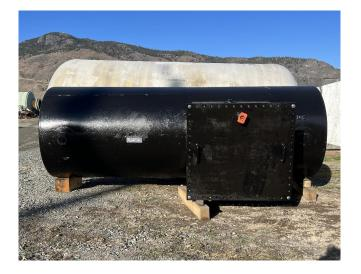
4,500 Liter Steel Buriable Double Wall Fuel Tank
