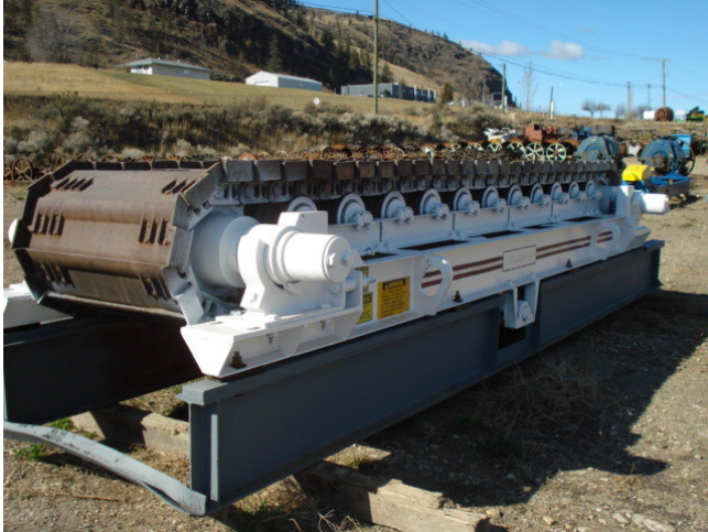
36 inch x 15 foot Telsmith apron feeders. Mounted on steel frame.
