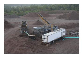
350 Ton Per Hour Classifying Plant. 10 ft. x 40 ft. Greystone Portable Classifier with Twin 44 in. Screws. Powerscreen Commander 1400 Screen. 120 HP Fresh Water Pump.
