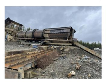
300 TPH 8ft Dia. x 42ft Long Scrubber Trommel Wash Plant
