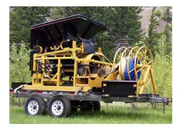
30 inch dia. x 78 inch long portable trommel. With feed hopper and sluice box. Tandem axle trailer and power generator.
