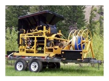
30 inch dia. x 78 inch long portable trommel. With feed hopper and sluice box. Tandem axle trailer and power generator.
