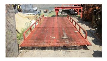
30,000 lb. Capacity Long Loading Ramp. 8 ft. Wide x 30 Ft. Long. 20 ft. Sloping Ramp Section. Landing Gear at one end for Additional Height Adjustment.
