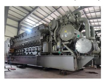
3,600kW EMD Diesel Generators
