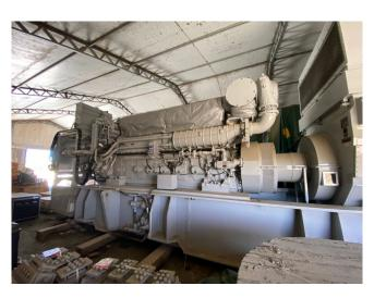
(3) 2200kW Caterpillar C280-8 Offshore Generators
