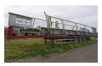
2m x 16m 24-Ton Steel Beam Pedestrian Bridge
